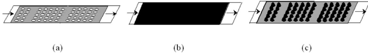
Figure 1. Schematic illustration of the successive steps involved in CDC. a) Support masked with lyophobic pattern. b) Over-coating of target solution. c) De-wetting of solution into lyophilic regions.
