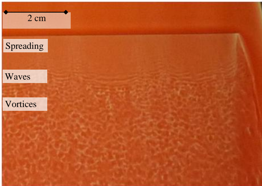
Figure 4: Shear wave instability by red Cyclopentanone on light blue Ethylene Glycol. Different characteristic areas from spreading to vortices are labeled (own figure).
