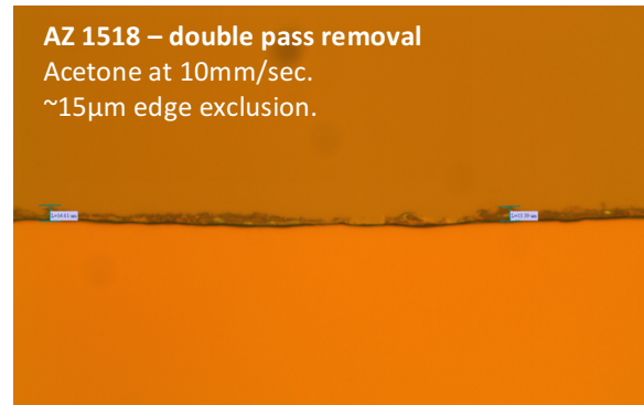
Figure 9: Double Pass Removal
