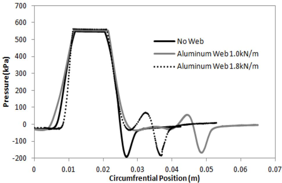
Figure 7. Measured pressure distribution in a laboratory device that had a tensioned web.
