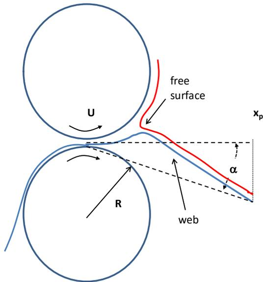
Figure 1. Configuration at the exit of a forward roll coating nip. The web can deform before the coating layer splits.  $\alpha$  is the take off angle of the web and  $x_p$  is the distance away from the nip that this point is applied. The center of the nip is taken as  $x=0$ .
