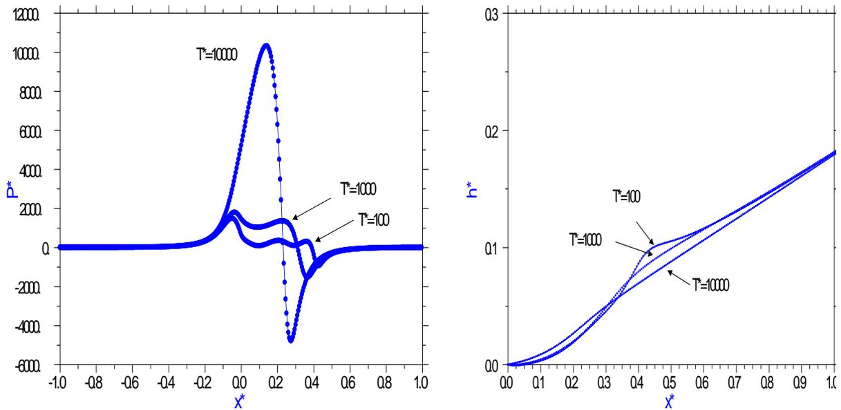
Figure 6. Same as Fig. 5 but for a negative angle of  $20^\circ$ , with the web being pulled upward from the nip. Left side is the pressure distribution and the right side is the web trajectories.
