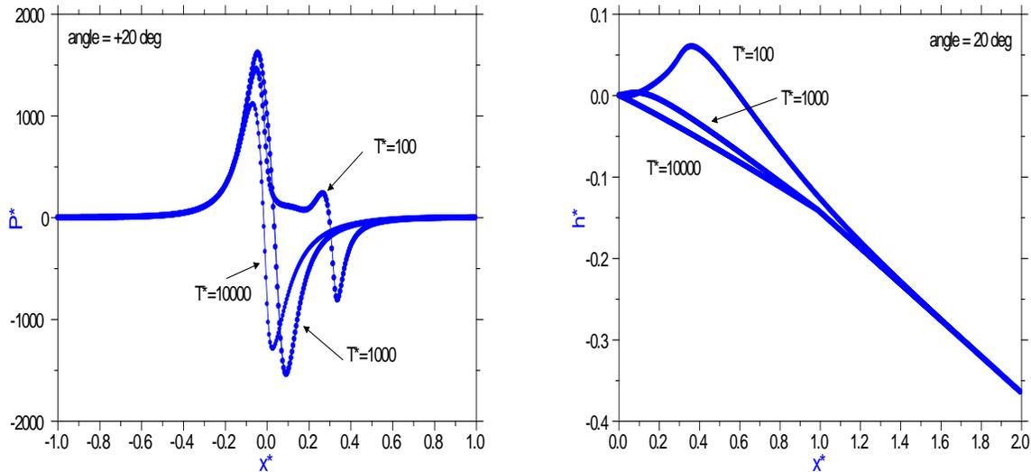
Figure 5. Results for positive (downward) take off angle of  $20^\circ$ , with the take up point being  $x_p^* = 2.0$  for  $h_i^* = 0.01$ . Pressure profiles are shown on the left. Web trajectories on the right.
