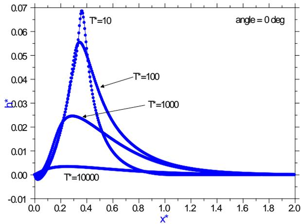
Figure 3. Web trajectories for various tensions when the web is pulled straight from the nip for various tensions and  $x_p^* = 2$ . Note that the y-axis is enlarged compared to the x axis.
