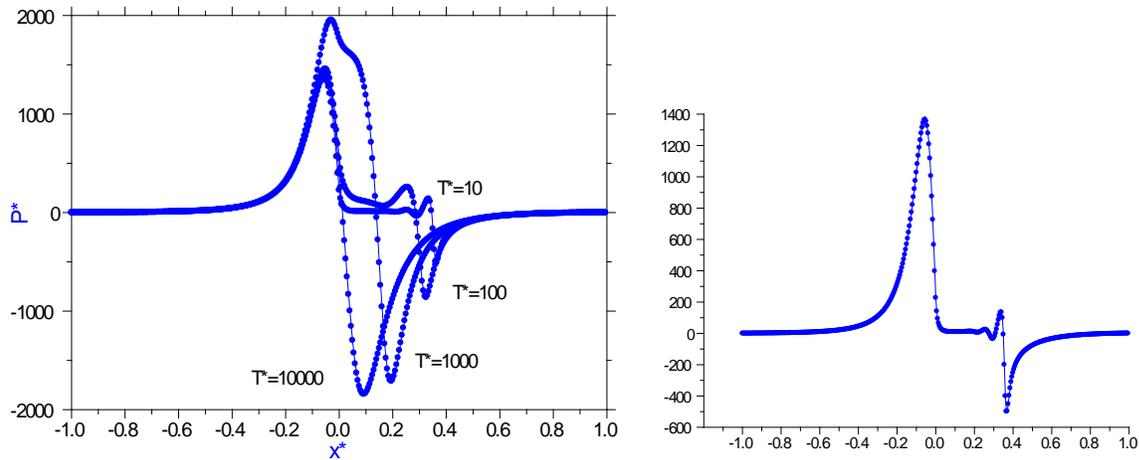
Figure 2. The pressure distribution predicted when the web is pulled straight from the nip for various tensions for  $h_i^*=0.01$  and  $x_p^*=2.0$ . On the right, the case for  $T^*=10$  by itself for clarity.
