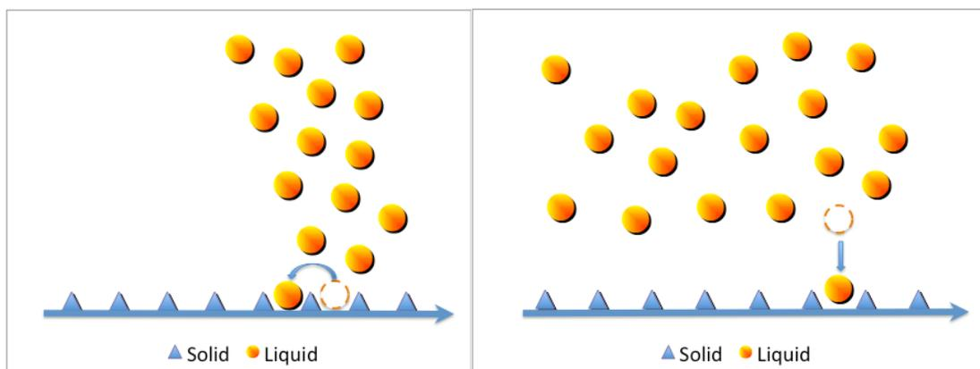
Figure 1 – Mechanism of dynamic wetting used for the MKT (left) and observed in molecular dynamics (right)
