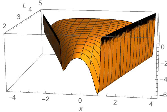
Figure 2 – Mie potential with  $n=3$ ,  $m=9$ ,  $A_l=5$ ,  $A_s=10$ ,  $B_l=3$ ,  $B_s=6$  with the liquid surface at  $x=-L$  and the solid surface at  $x=+L$ .
