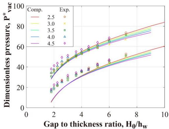
**Figure 4.** Computational (line) and experimental (marker) coating window at different roll speed (unit: mpm).
