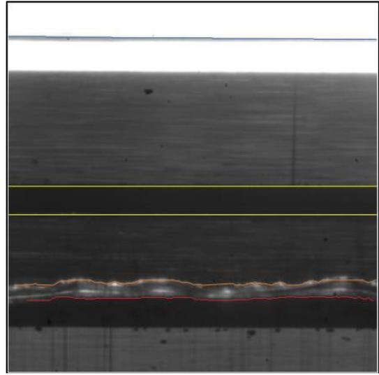
**Figure 3.** The result of image analysis. The red, orange, yellow and blue lines are SCL, DCL, feed slot and downstream meniscus location, respectively.
