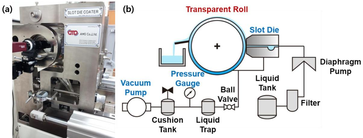
Figure 1. (a) An image of experimental set-up with CCD camera, and (b) a schematic diagram of the slot coating device.
