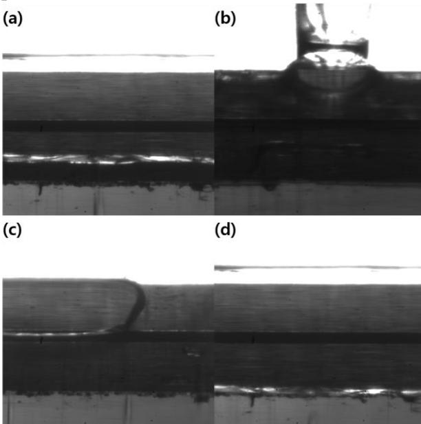
Figure 2. Examples of the visualized coating bead flow at: (a) stable condition, (b) low-flow limit, (c) bead break-up limit, and (d) weeping limit.
