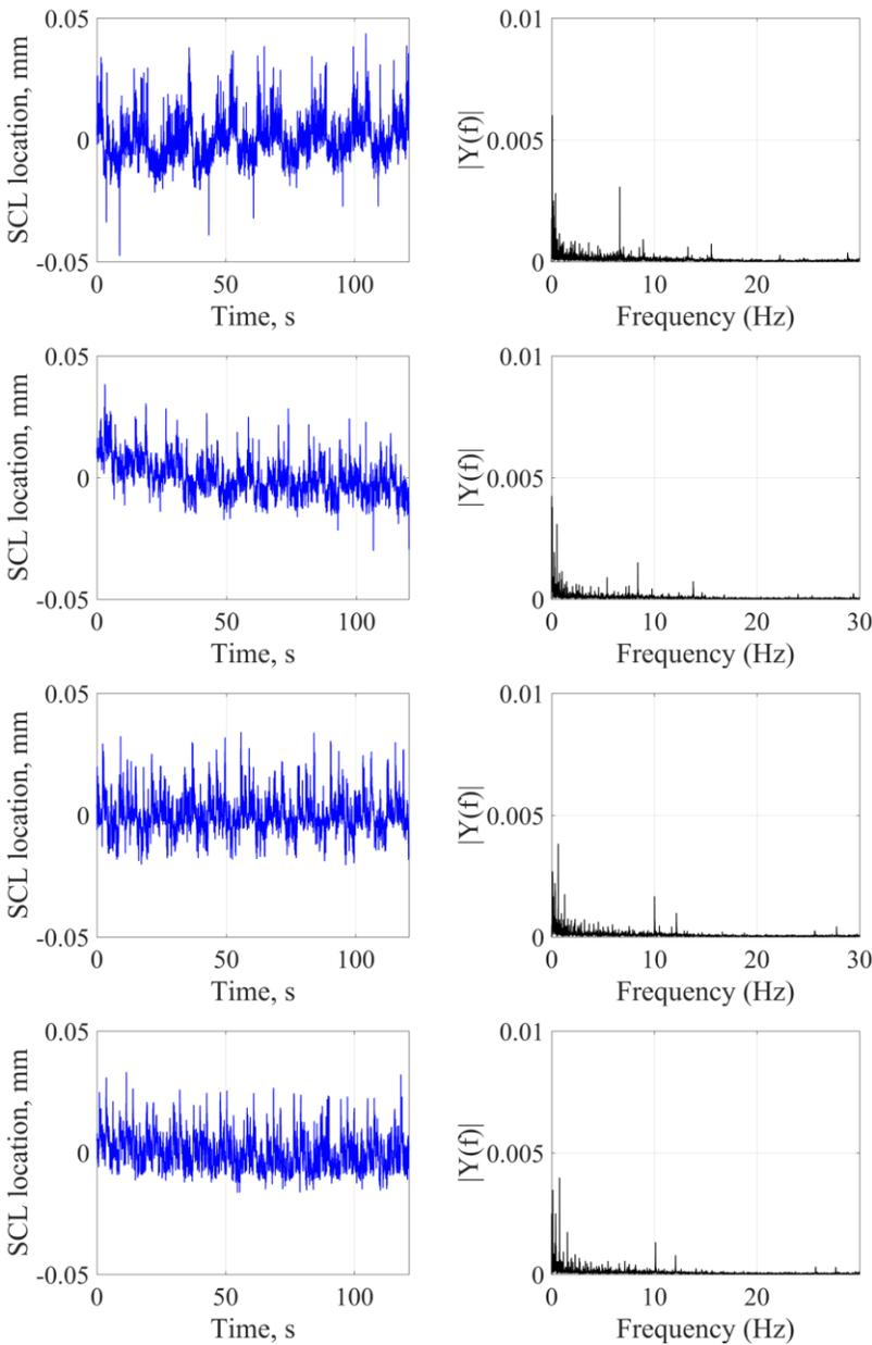
**Figure 5. Relative SCL location to the initial location with respect to time (left) and FFT results (right). The roll speed is 1.5, 2.0, 2.5, and 3.0mpm, respectively in downward direction.**
