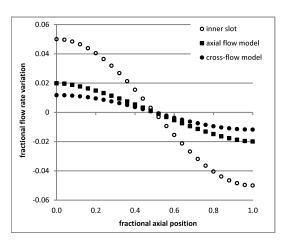
The biggest deficiency of the axial flow model occurs in cases where there is little axial flow as a result of a good flow distribution in the primary slot. As the chart shows for the conditions of the second
