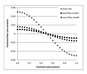
The second example is for a highly shear-thinning, viscous liquid. In this case the cross-flow model predicts a better flow distribution than the axial flow model. The axial flow model does not consider the viscosity reduction caused by the cross flow. In extreme situations of purely viscous flow, where axial
