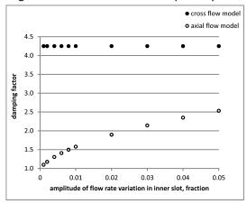
example, the axial flow model predicts little improvement of flow distribution in this case because the shear-thinning effect of the cross flow is not considered. A small axial flow rate gives a high viscosity.
