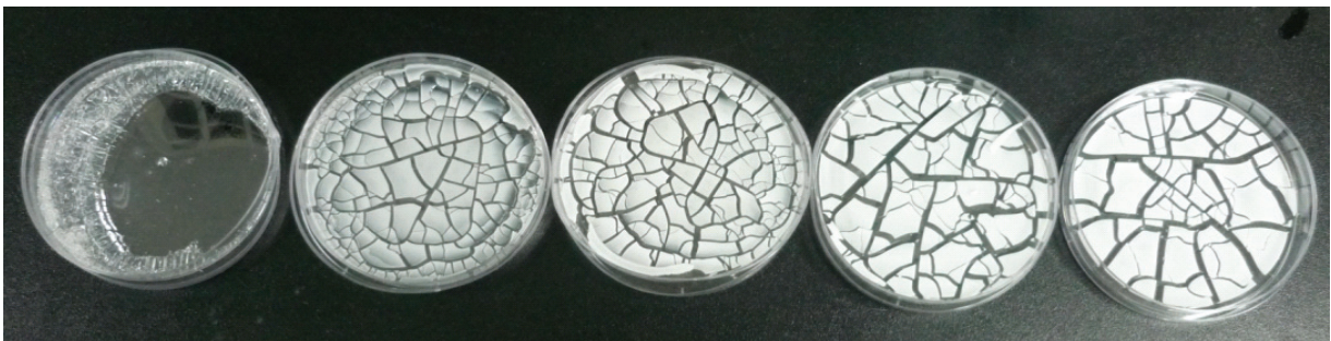
Figure 2. Crack Behavior of Ludox SM with increasing NaCl concentration from 0M to 0.12M
