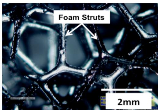
Figure 1 Optical microscope image of carbon foam with 10 pores per inch (10 PPI).
