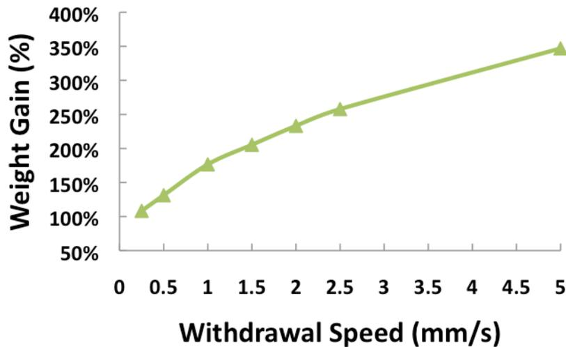
Figure 2 Effect of withdrawal speed on final weight gain for a 10PPI foam coated with a solution of 90 wt% glycerol and 10wt% water.
