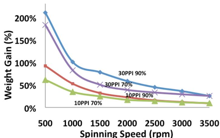
Figure 5. Effect of spinning speed on weight gain for different foams and coating solutions and the spinning time is 15 seconds.
