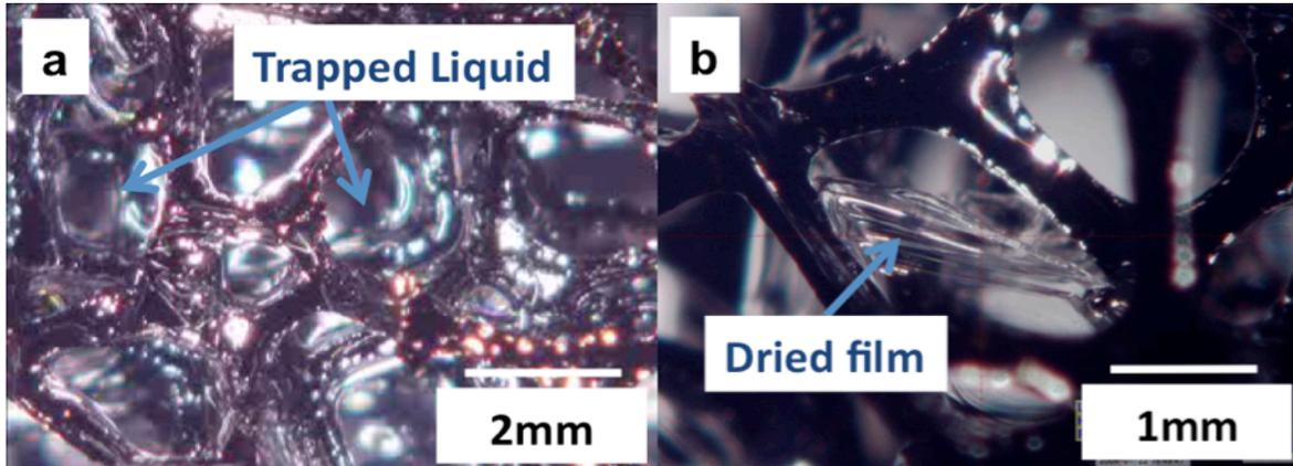
Figure 3 Optical microscope image of (a) liquid trapped within carbon foam pores (10PPI) and (b) dried coating (alumina) trapped in the pore space.
