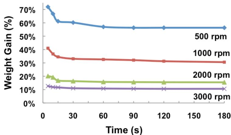
Figure 4 Effect of spinning treatment and speed on weight gain for a 10PPI foam coated with a solution of 70wt% glycerol and 30wt% water.
