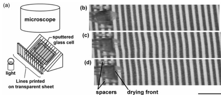
Figure 3. (a) Schematic illustration for reflection image observation. Reflected images (b) right after injection of colloidal suspension, (c) just before perpendicular crack formation and (d) 10 s after (c). The aspect ratio of each image of (b) – (d) was intentionally changed from the original ratio of 1 : 1.6 to 1 : 5 to highlight the distorted reflection image of parallel lines. The scale bar is 2 mm in each direction.
