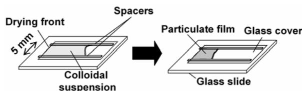
Figure 1. Schematic illustration of handmade glass chip used in our study.
