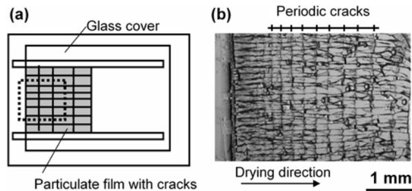
Figure 2. Typical example of formed cracks. (a) an overview of formed colloidal film with cracks. (b) is optical microscope image of the dotted square in (a).
