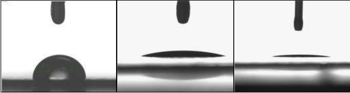
**Figure 1.** Solvent contact angle and absorption on the MPL layer of a GDM substrate. (left) EtOH:H<sub>2</sub>O::3:2 w/w, 26.2 mN/m, 93.4° after 1sec; (center) nPrOH:H<sub>2</sub>O::3:1 w/w, 24.2 mN/m, 14.4° after 1sec; (right) nPrOH:H<sub>2</sub>O::3:1 w/w, 7.1° after 5sec.
