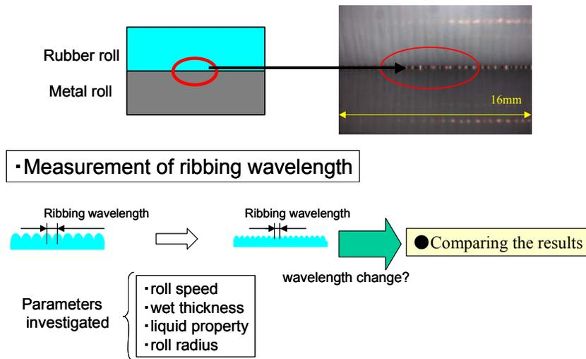
Fig.2 Example of roll coating visualization and data extracted from image
