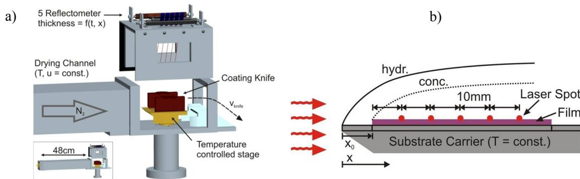
Fig. 1: a) Schematic drawing of the drying channel with integrated knife coater and linear array of five monochromatic reflectometers. The inset shows the 40 cm long channel for airflow distribution in front of the coating stage. b) illustrates the position of the film at the stage and the laser spots for thickness measurement.
