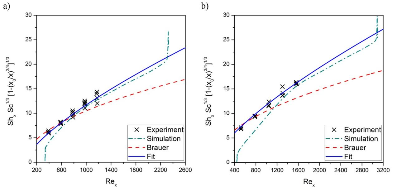
Fig. 2: Comparison of the numerical and experimental Sherwood numbers with the analytically derived correlation [5] and the adapted correlation [2] at different mean velocities a)  $u_0 = 0,3 \text{ m/s}$  and b)  $u_0 = 0,4 \text{ m/s}$ .
