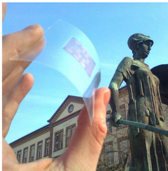
Figure 1: Polymer based hybrid solar cell, coated on a flexible PET Substrate
