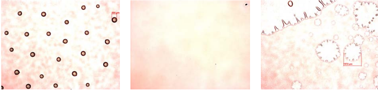
Figure 1: Hole injection layer (small molecule) prepared by dropcasting and dried under different conditions. Left: Solved in Dioxane, Middle: Solvent mixture, fast drying, Right: Solvent mixture, slow drying.
