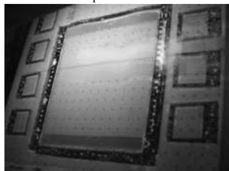
Figure 9: Slot die coated PEDOT:PSS and LEP layers, patterned by surface energy
