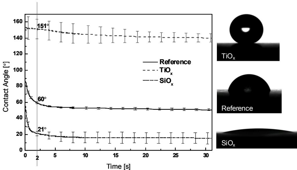
Figure 1: Water contact angle (CA) for reference (solid), TiO<sub>x</sub> (dash) and SiO<sub>x</sub> (dash dot) coatings as a function of time. The subfigures to the right display the captured images from the measurement at the 2.0 s. The error bars display standard deviations from three measurements.
