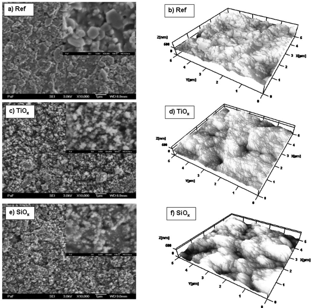
Figure 2: SEM (to the left) and AFM (to the right) images of the reference sample a, b), TiO<sub>x</sub> nanoparticle coating c, d) and SiO<sub>x</sub> nanoparticle coating e, f).
