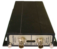
After: 2 channel enclosure with USB power/data output
