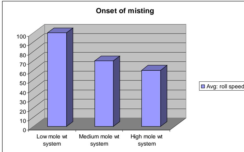
Fig. 2: Onset of misting with molecular weight of coating
