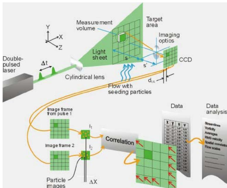
Figure 5: Particle Image Velocimetry Method.
