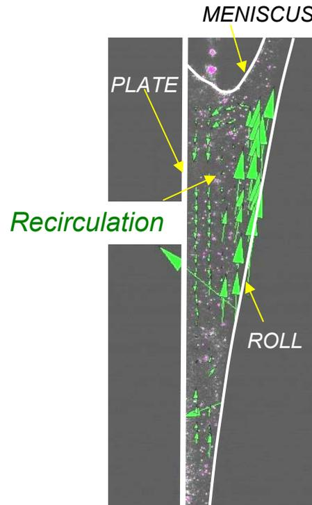
Figure 6: Lateral view with measurement of velocity field,
