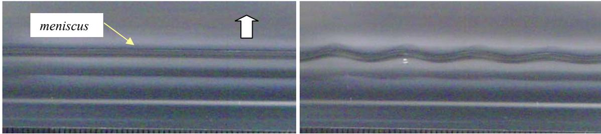
Figure 4: Frontal view of coating bead at  $H_0 / R = 3 \times 10^{-3}$  and (a)  $Ca = 0.6$  and (b)  $Ca = 0.65$
