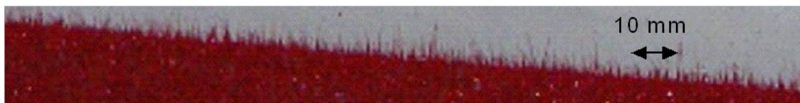
Figure 1. View of the roll surface 90o away from nip exit showing numerous ink filaments being extended and thinned due to centrifugal forces.
