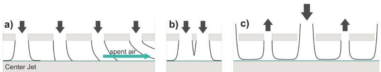
**Fig. 2:** Interaction effects appearing in arrays of impinging jets. Cross-flow effect a), merging of jets pre-impingement b), spent fluid removal pre-interaction over the orifice plate c).
