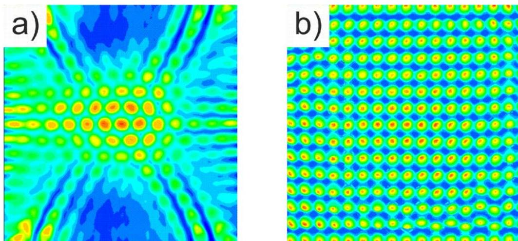
**Fig. 1:** Qualitative prediction of the distribution of the heat transfer coefficient by transient heat transfer experiments for a confined staggered array of impinging jets (a), qualitative prediction of the distribution of the heat transfer coefficient by transient heat transfer experiments for a confined inline array of impinging jets with local removal of the spent fluid (b).
