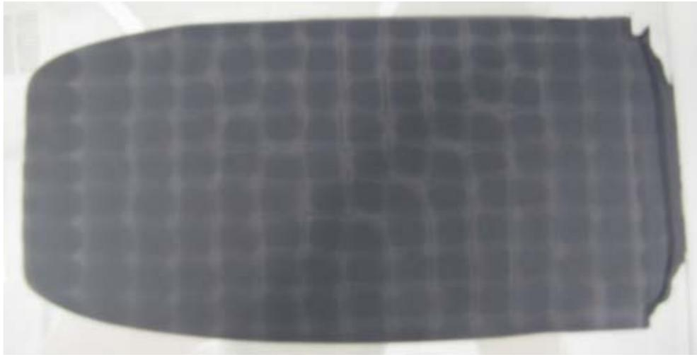
**Fig. 3: Anode for Li-ion Battery dried under an inline array of impinging jets. The coating shows an unwanted patterning throughout the film due to the inhomogeneous drying conditions.**
