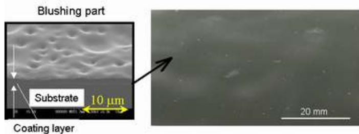
**Figure 1 Coated film with blushing defect**
