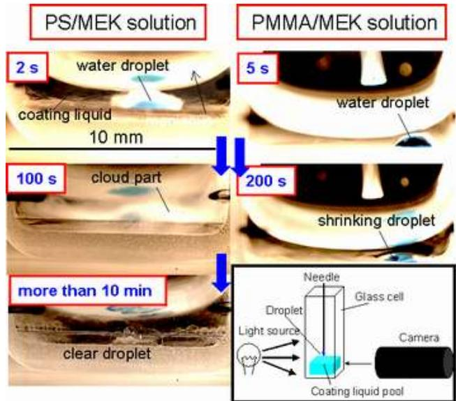
Figure 4 Water dissolution behaviors in each solution (left: PS/MEK, right: PMMA/MEK)
