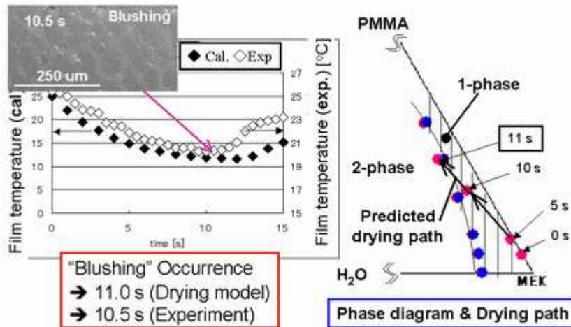
**Figure 6 Comparison between the calculation and the experiment result (PMMA/MEK system; 68RH%, 0.5 m/s, 25 °C)**
