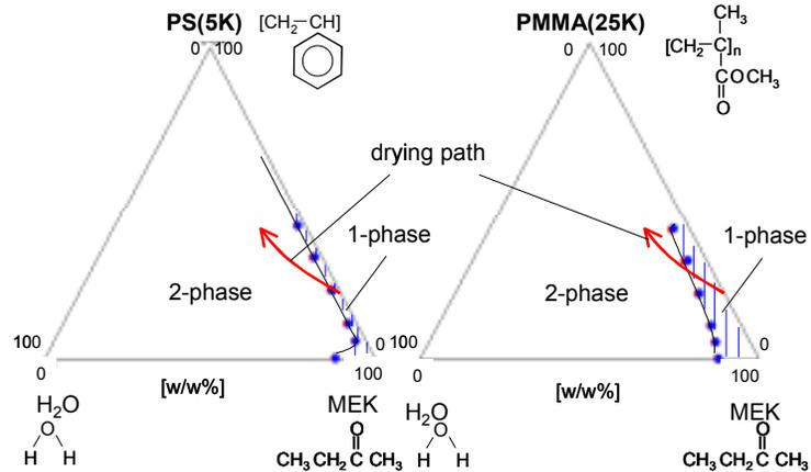
**Figure 5 Phase diagrams of ternary systems (Polymer-H<sub>2</sub>O-MEK)**
