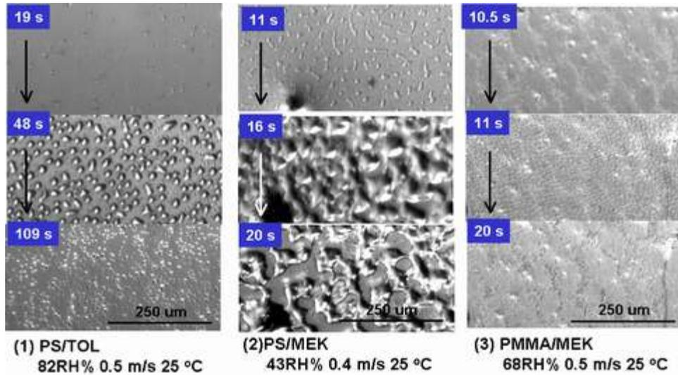
Figure 3 Surface deformations in each system
