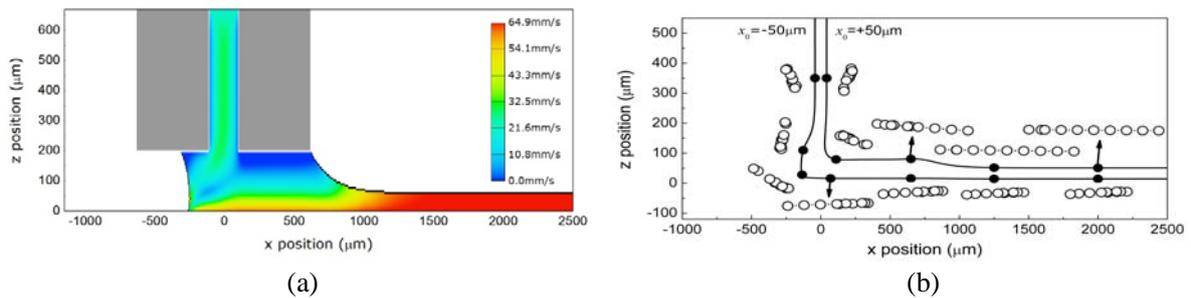
**Figure 1.** (a) Velocity magnitude contour under the operating conditions considered in this study. (b) Conformational change of around polymer molecule along different streamlines in the slot coating flow.
