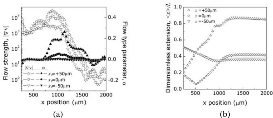
**Figure 2.** (a) The changes of flow strength ( $\nabla v$ ) and flow type parameter ( $\alpha$ ) around polymer chains entered at three different positions and (b) the change of extension ( $\langle x \rangle / L$ ) of each molecule along the flow directions ( $x$ ).
