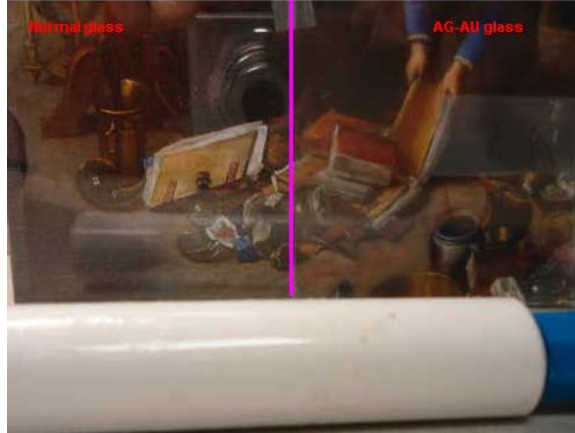
Figure 14. Image of a white pencil on AG-AU glass (right) and normal glass (left). The distance of color picture from AG-AU and normal glass is approximately 2 cm.
