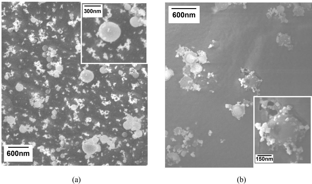
Figure 1. Cryo-SEM images of ATO/latex dispersion (a) and ITO/latex dispersion (b).
