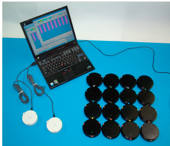
Figure 2: Sixteen-channel system showing gap discs, RF signal receivers (in white) and individual gap results shown on custom software
