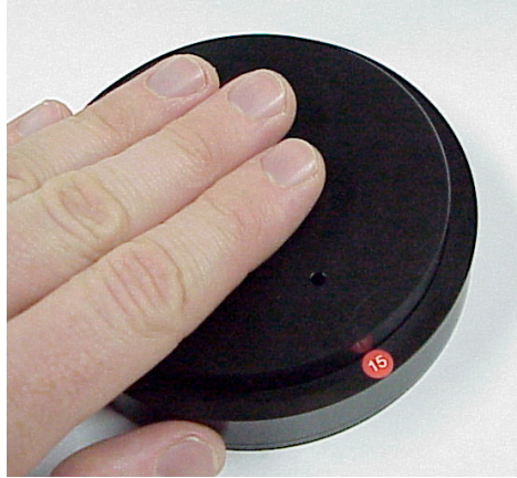
Figure 1: Pressure applied to the spring-loaded enclosure is transferred to a non-contact displacement sensor, which calculates the nominal gap.
