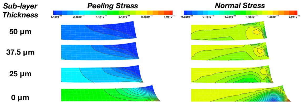
Figure 2: *Principal stresses in the upper layer of a solidified, fully dried two-layer coating( sub-layer not shown). Edge retraction grows with rising sub-layer thickness but is limited to near-edge.*
