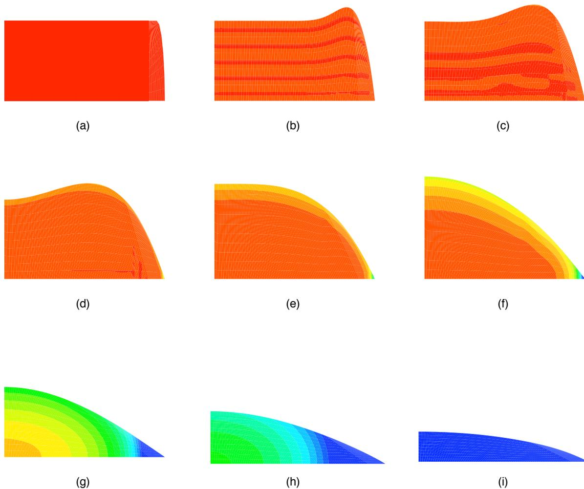
Figure 3: *Edge shape of a still liquid coating at different times of drying. Thickness is magnified ten-fold for better resolution. Solidification starts at the edge and moves toward the center of the narrow stripe of coating.*
