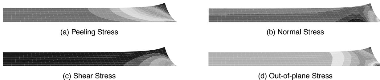
Figure 1: *Stresses near the edge of a single-layer fully dried coating. Stresses are highest near the edge and fall rapidly away from the edge; they are appreciable up to six thicknesses away.*
