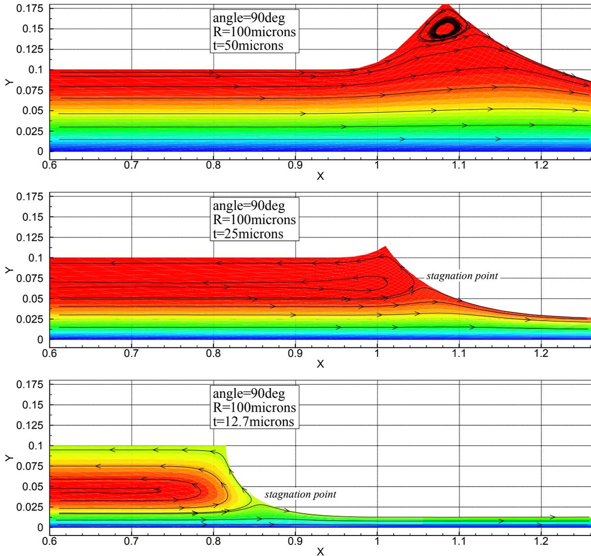
Figure 5: Evolution of the streamlines as the flow rate falls.
