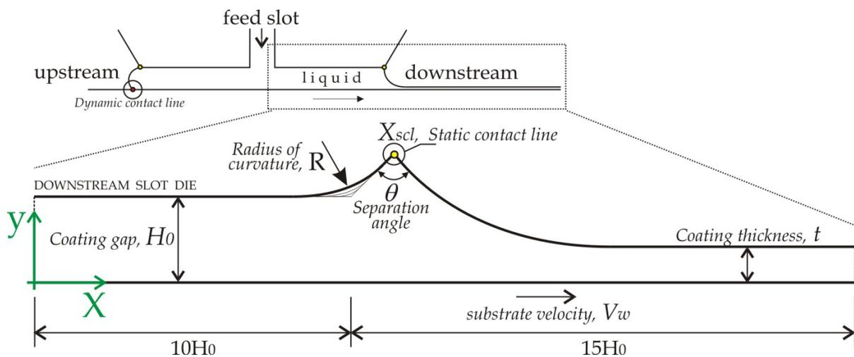
Figure 2: Sketch of the flow domain near the downstream free surface.
