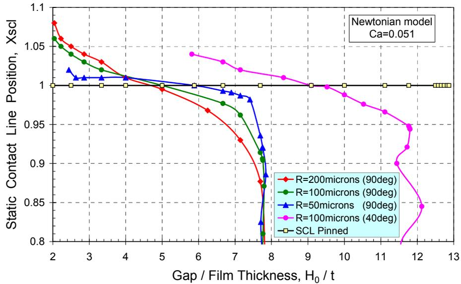
Figure 4: Static contact line position at different static contact angles and radius of curvature of the die corner.
