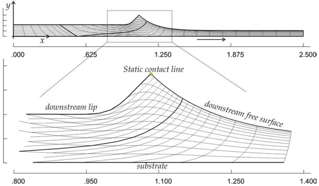
Figure 3: Sample mesh with 342 elements and 6854 degrees of freedom.
