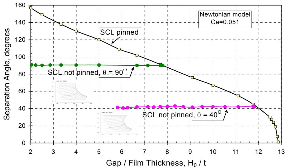
Figure 6: Contact angle as a function of gap-to-thickness ratio for pinned and free moving contact lines.
