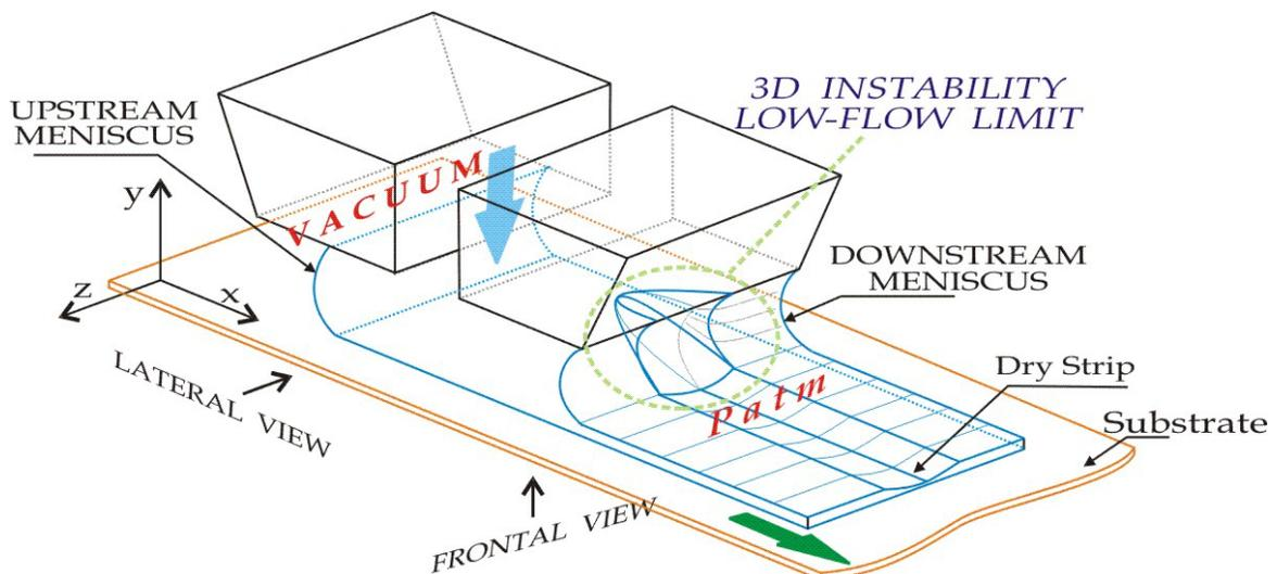
Figure 1: Sketch of the bead break-up from the upstream meniscus, which marks the onset of the low-flow limit in slot coating process.
