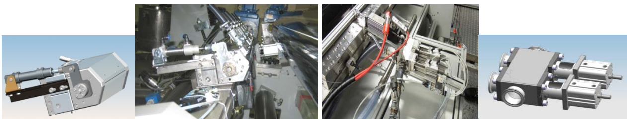
Picture 6: Intermittent coating with rotating bar in slot-die versus valve technology in front of slot-die
