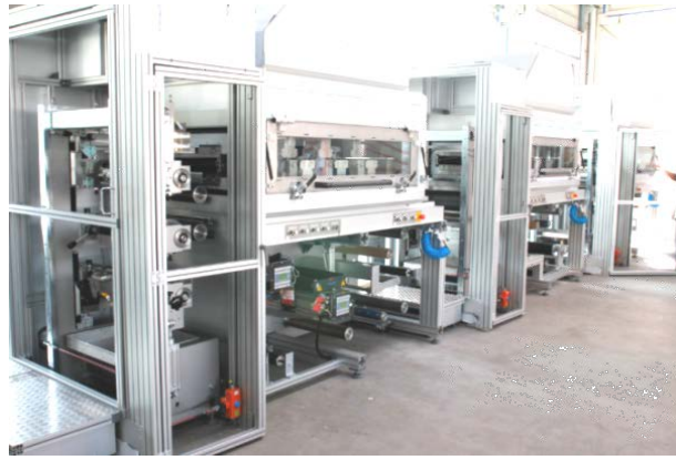
Picture 13: Roll to roll coating multi-head line for organic solar cell production
