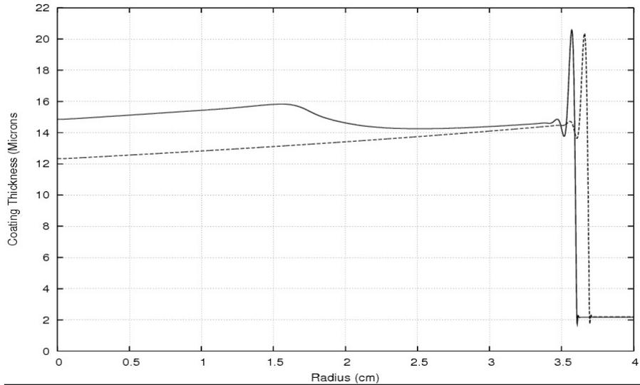
Figure 4: Two axisymmetric spin coating profiles. The dashed profile has 5 % of the coating deposited after the start of the motion. Liquid volume is 0.05 ml; the rotation rate is 700 rpm. Other parameter values are the same as for the previous case.
