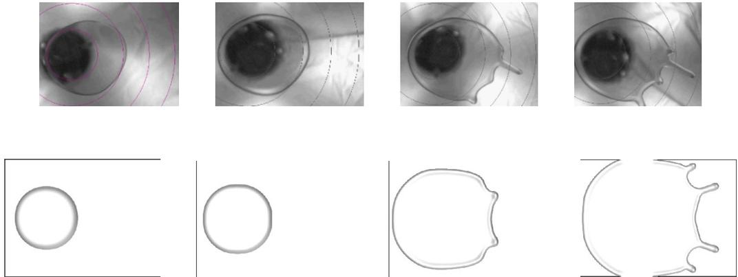
Figure 2: Early fingering caused by gross misalignment of initial drop in spin coating; experiment and simulation. Newtonian liquid is assumed in the simulation.
