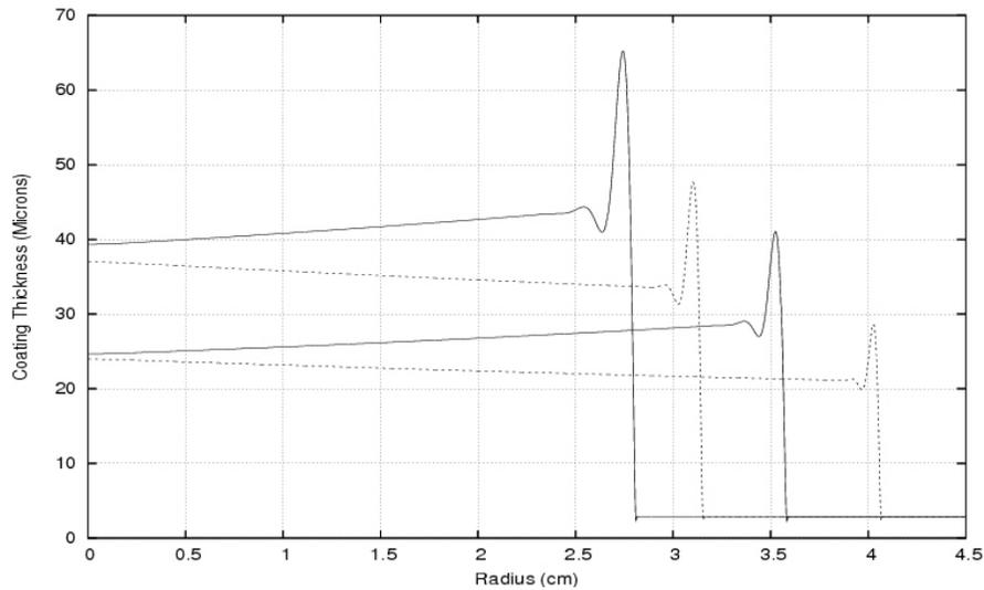
Figure 3: Calculated spin coating thickness profiles for optical lenses at two times. The rotation rate is 500 rpm, the viscosity is 2 centipoise, and the liquid volume is 0.1 ml. Results are shown for a a convex (solid) and a concave lens (dashed) at 0.4 sec and 1.0 seconds after the start of spinning. The lens radius of curvature is 16.5 cm, corresponding to an optical “strength” of 3 diopters.
