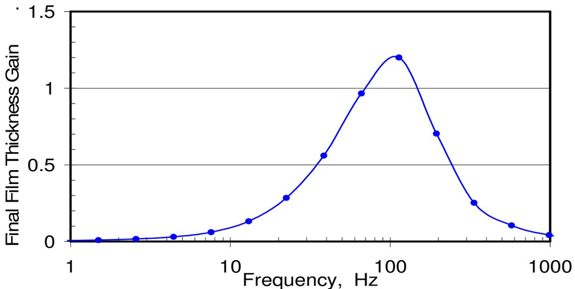
Fig. 4 Example of frequency response to coating gap oscillation. The web velocity is 50cm/s; both layers have the same density, 1.0 g/cc and the same viscosity, 0.5 P; at the top layer/air interfacial surface tension is 50dyn/cm; the vacuum pressure is 0 Pa; the film thickness ratio (upper to lower layer) is 0.5; the Peclet number is  $10^5$ .
