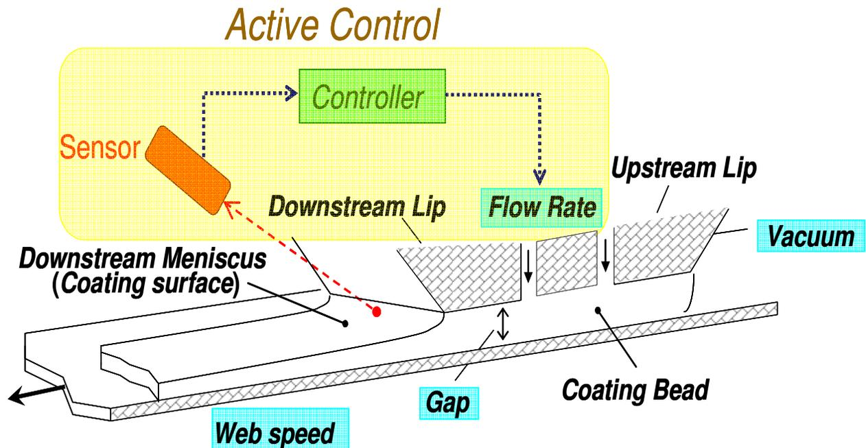
Fig. 5 Active control of two-layer slot coating flow
