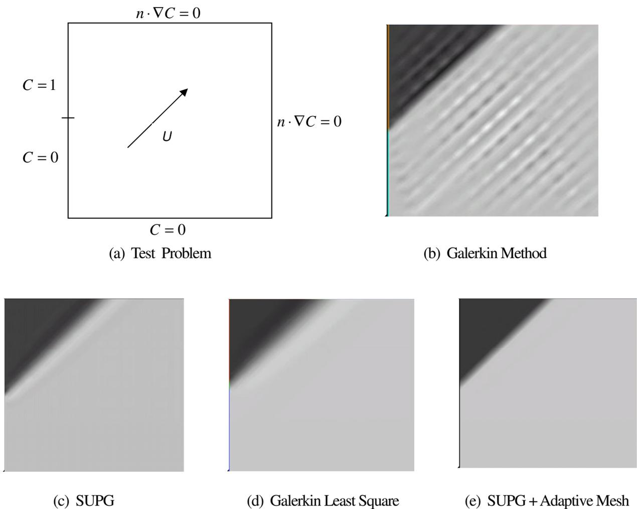
Fig.2 The sequence of alternatives tested. Conditions: 961(31 x 31) Quadratic Basis Functions, Peclet Number,  $10^5$ . The separation point is located at intersection of  $C=0$  and  $C=1$  in Fig. 2(a).
