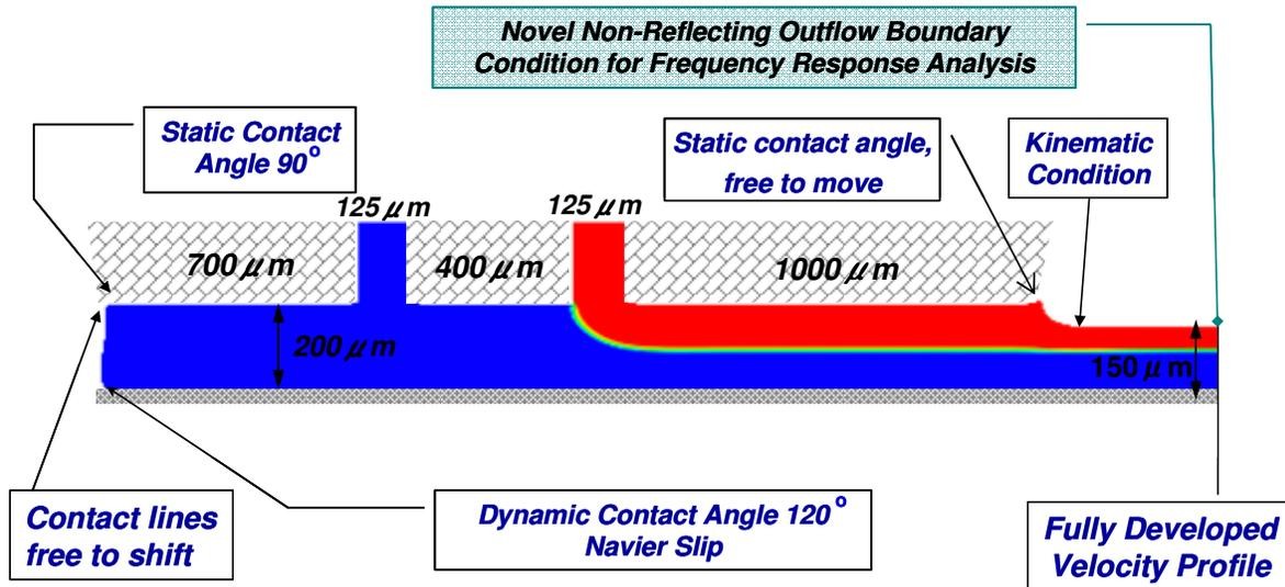
Fig. 3 Boundary conditions and a predicted steady state.
