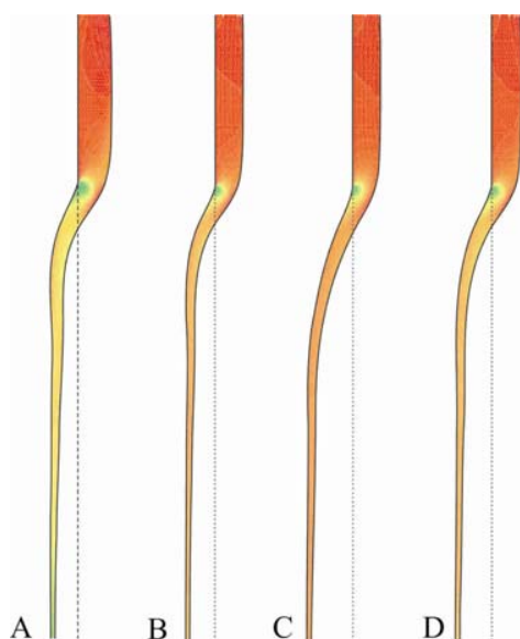
Figure 1 Teapot effect for different coating fluid rheologies (Adhesive A-D): horizontal deflection of the curtain. Color contour: pressure field (red: atmospheric pressure, blue/green: low pressure region, Re = 5 )
