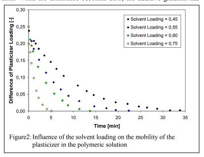
Goal of these experiments is to get reliable data to be able to describe the diffusion of non-volatile components in polymeric systems and implement this information in simulation to describe the inhomogeneous distribution of the non-volatile components in the final foil.
