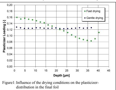
To be able to describe the drying process and to explain inhomogeneous distribution of non-volatile components in the final foil, the diffusion of the solvent in the polymeric solution must be taken into account as well as the mobility (i.e. the diffusion) of the non-volatile additive. For a correct simulation
