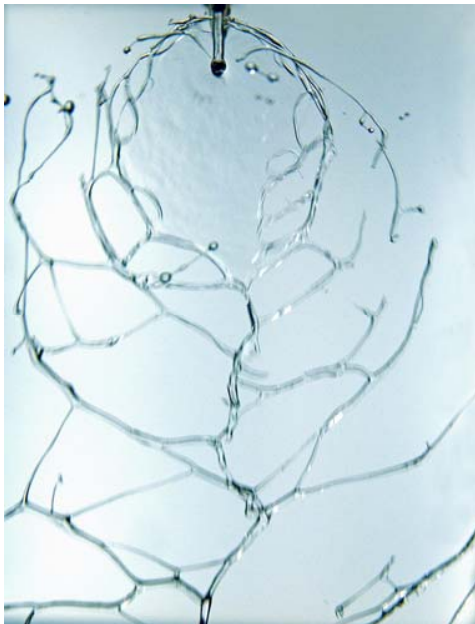
Figure 1: High speed photographs of the fluid sheets formed by impinging jets of 25mM CTAB/NaSal at 6.2m/s.
