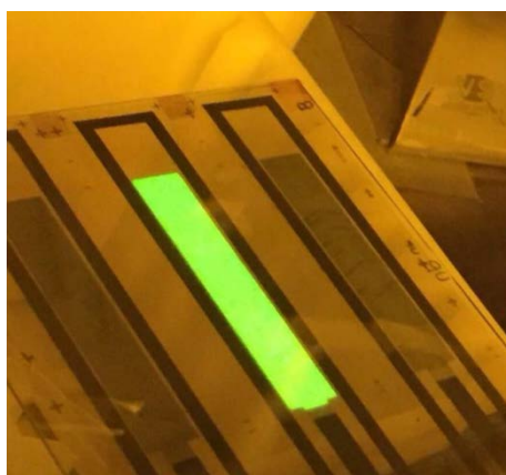
Figure 5. Bottom-emissive OLED on plastic barrier foil
