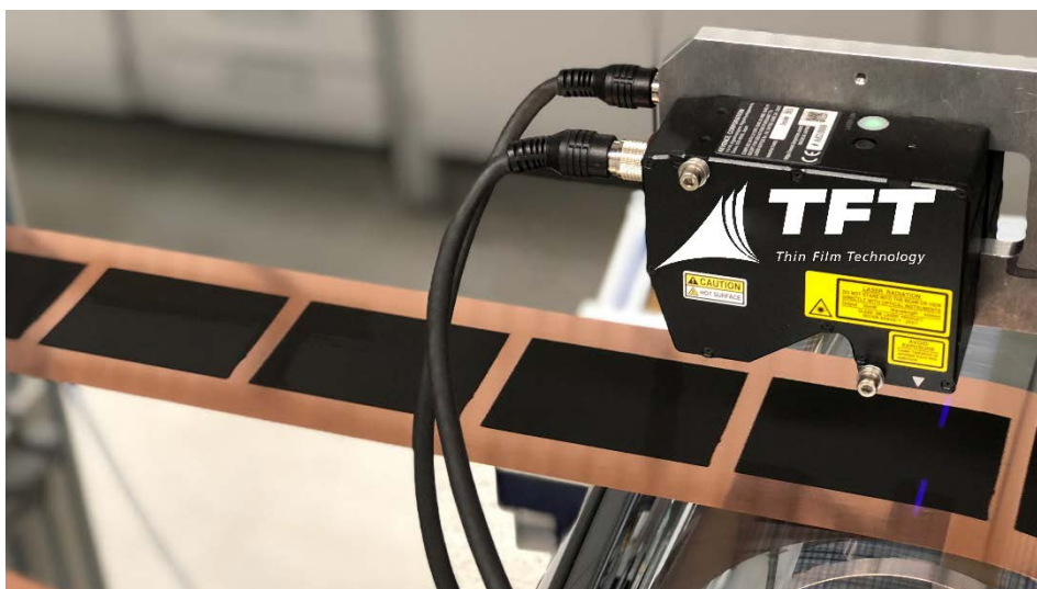
Figure 1: Anode film with 80 mm coated patterns and 20 mm non coated intersections between the patterns.
