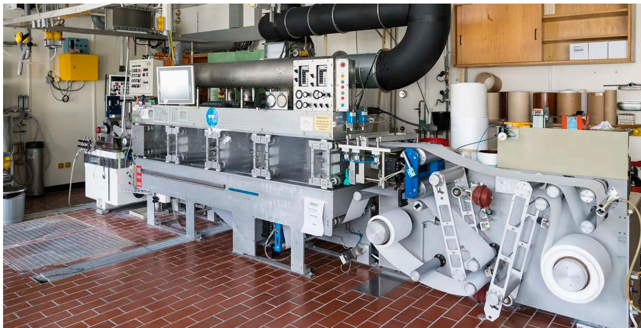
Figure 8. DEXMA Loop- machine for curtain coating [iPrint institute, Switzerland]
