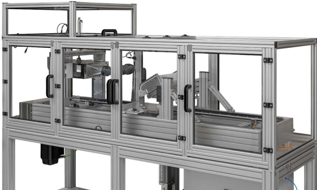
Figure 7. TSE TableCoater for curtain coating [TSE Troller AG, Switzerland]
