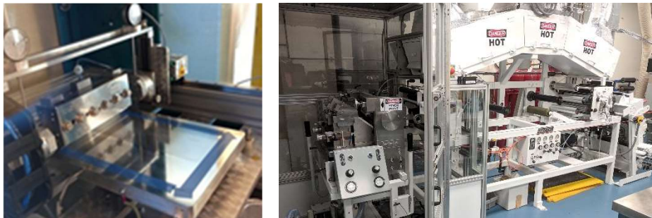
Figure 3. (left) Batch coater used for initial formulation adjustments and (right) small pilot coater used for 2-layer slot and multi-layer slide trials.
