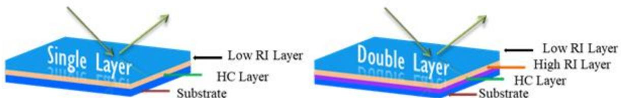
Figure 1. Anti-reflective Coating Structure
